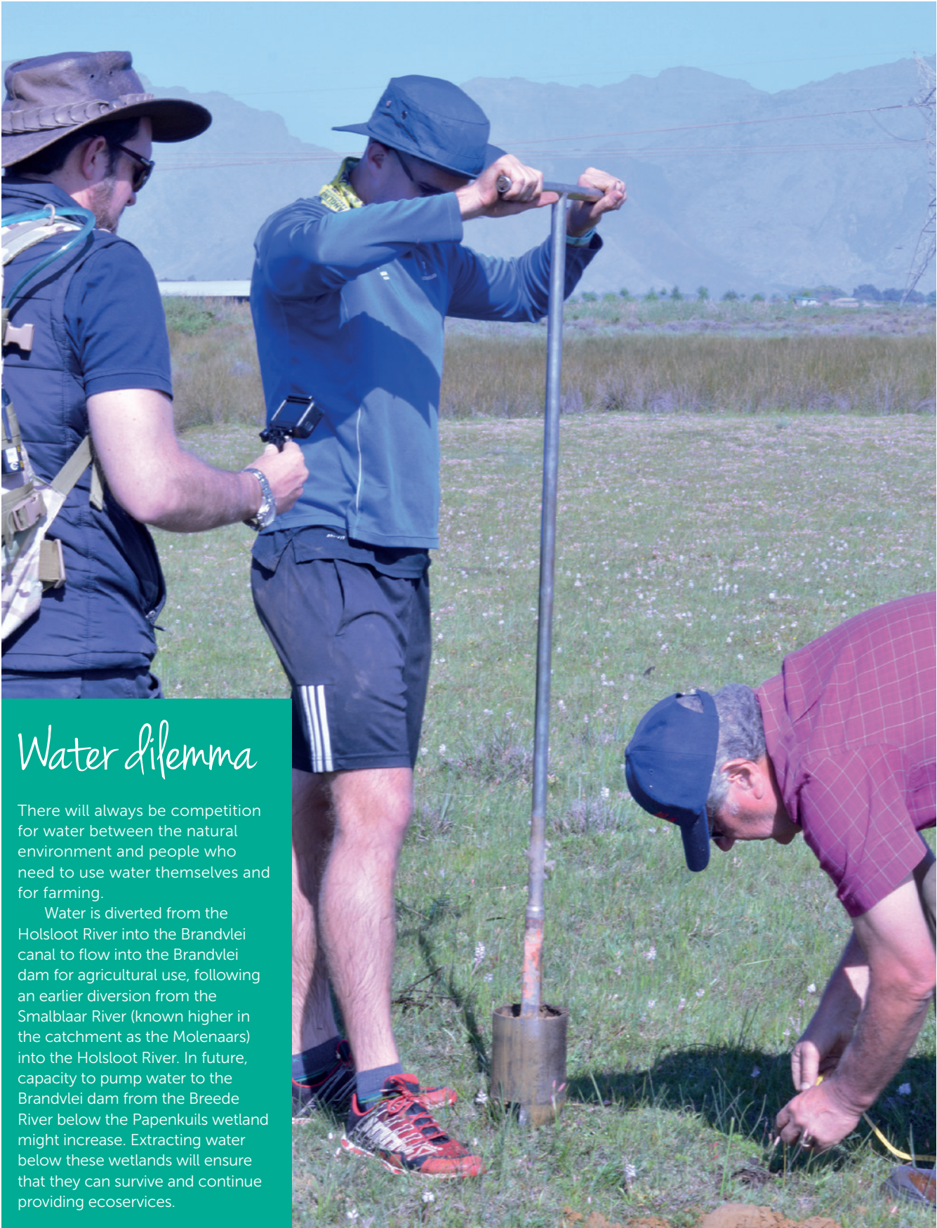
Phil McLean, Zahn van Wyngaard and SRK's Simon Lorentz work an auger to sample soil along the transect to understand soil characteristics linked to the plant communities and wetlands.
