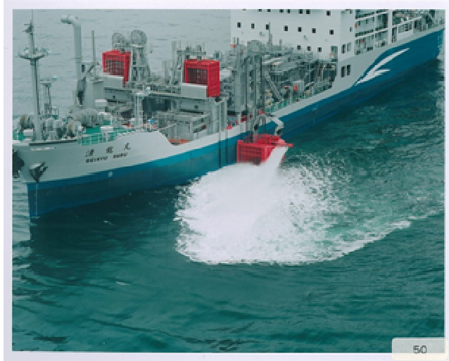
Photo 3. Oil recovery system with water jet Oil collecting device
