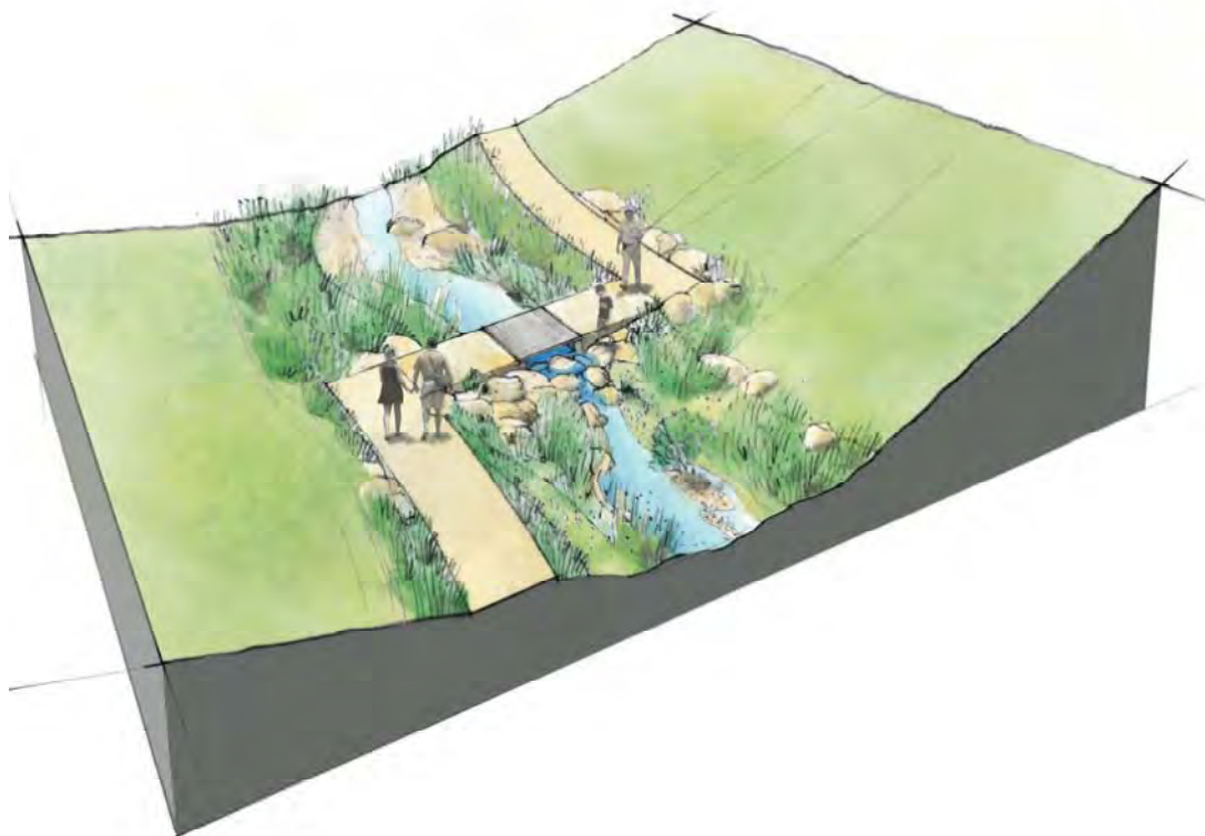
Figure 9. Example of Low Water Trail Crossing (Westside Creeks Restoration Project Conceptual Plan)
