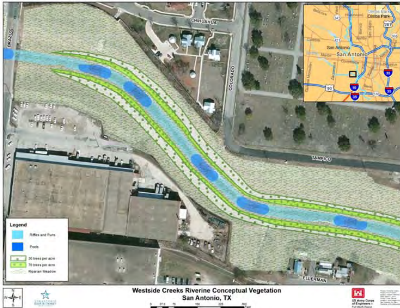
Figure 13. Representative Concept of Maximum Practicable Restoration for the Westside Creeks
