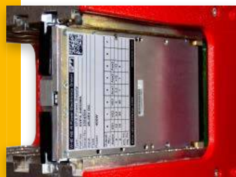
VPX340DMA back side with wedge lock
