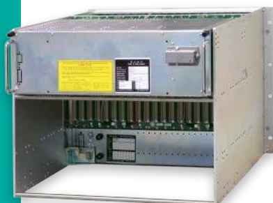
6U VME 6021 Crate rear side with power supply
