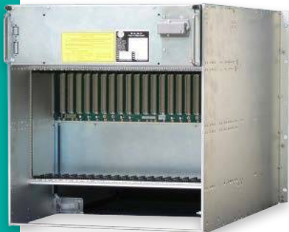
9U VME 6021 Crate rear side with power supply
