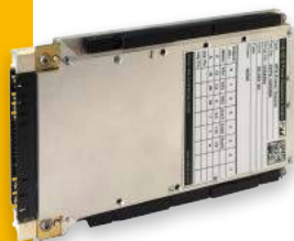
VPX340DMA back side with wedge lock
