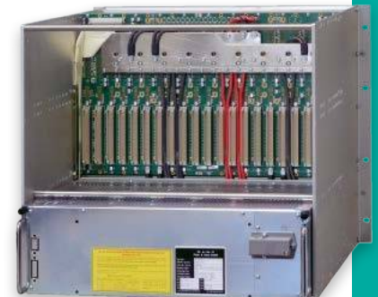
6U VME 6023 Crate rear side with power supply
