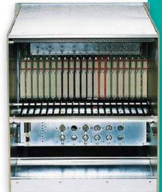
6U VME 6023x JLAB Crate rear side without power supply
