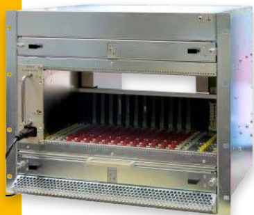
MTCA chassis with MTCA4 power supply
