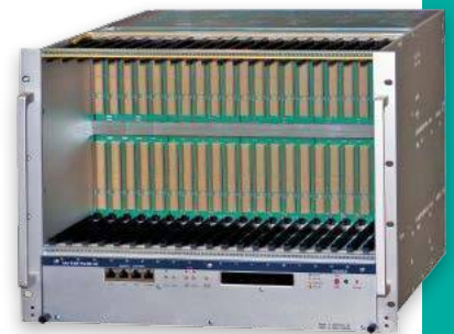
6U cPCI 6021 Crate outfitted with four 5-slot 6U backplanes
