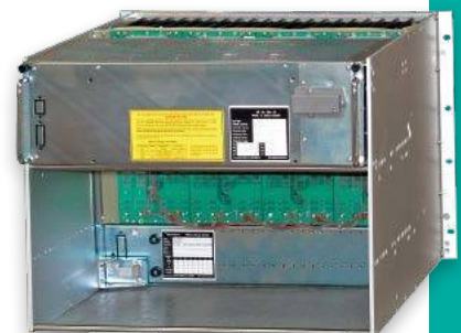
6U cPCI 6021 Crate outfitted with four 5-slot 6U backplanes rear view
