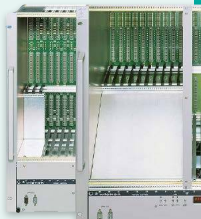
VARIO divider option (version 1 left, version 2 right)
