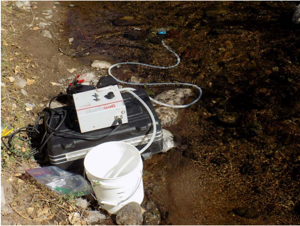
Figure 5. Sampling apparatus for collection of eDNA samples.
