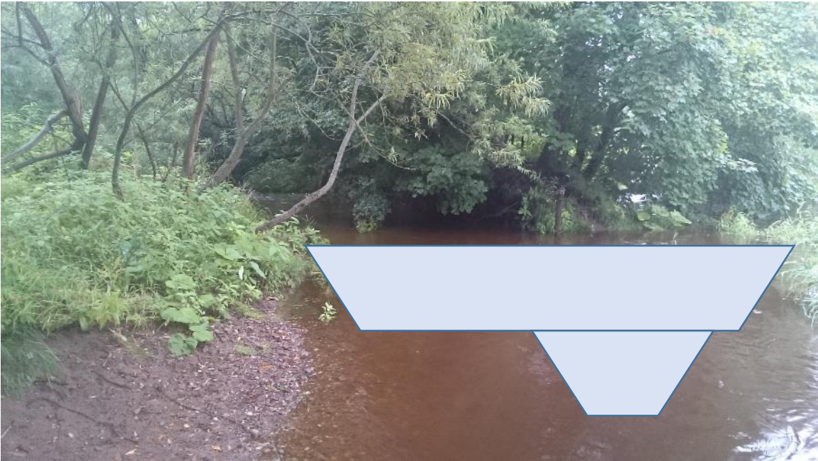
Figure 9. The ephemeral side channel (in high flow) as it re-joins the Wharfe d/s of Beanlands Island. Overlaid is a schematic of a two-stage channel. As seen, the water fills the complete cross-sectional area, but in low flows, is focussed into the more appropriate, smaller dimensioned channel. Here, being on a bend, the deeper channel should be encouraged towards the outside bank as would naturally occur.
