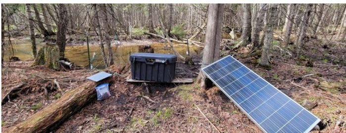
Figure 3. Upstream PIT array at Lower Nejedlo Rd crossing, installed downstream of crossing. Image of the Nejedlo PIT monitoring system from the right bank (top) and the left bank (bottom).
