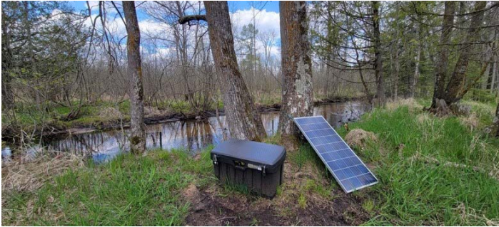
Figure 2. Downstream PIT array at McMahon Rd crossing, downstream of the crossing. The multi-reader, auto-tuners and deep-cycle marine batteries are located within the black locking box.
