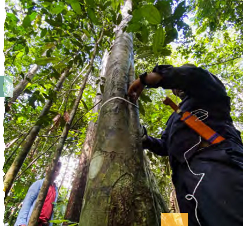
Figure 3 Diameter at breast height (DBH) is one of the most common dendrometric measurements of diameter of a standing tree. © Photo: Wilmar International
