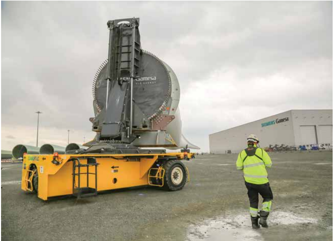
The COMBi-LC Blade load mover can either be driven by an operator or controlled remotely. (Courtesy: Combilift)
