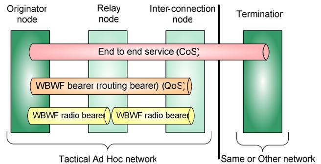
**Figure 1 – ETARE WBWF QoS Architecture**
