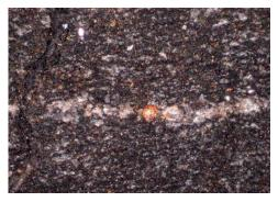
FIGURE 2. A RELATIVELY THICK BEDDING PLANE CONTAINED IN A SHALE FRAGMENT IS PICTURED. A BRASSY YELLOW PARTICLE COMPOSED OF IRON SULFIDE IS LOCATED WITH THE RELATIVELY THICK WHITE LAYER.
