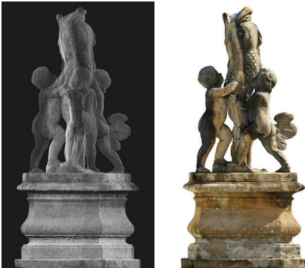
Figure 2. Laser scanning survey of the sculpture group in the Malta Fountain. Left: cloud point image. Right: 3-D rendering.
