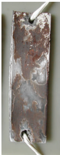
Figure 4. Appearance of a sensitized sample B after a 15-month exposure to an outdoor “severe” environment.
