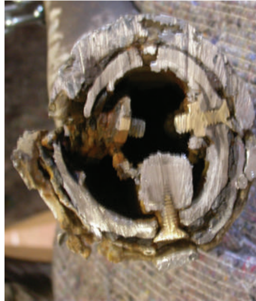
Figure 6. Set of screws found in the arm of Autumn , presumably from former repairs.
