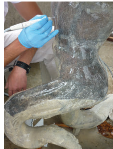
Figure 15. Removal of calcareous concretions on one of the lead sculptures using ultrasound.
