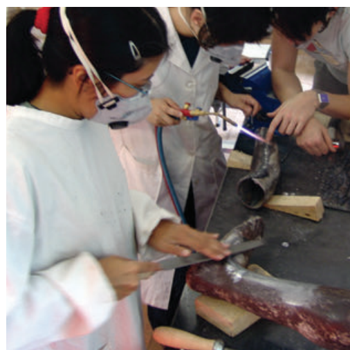
Figure 10. Finishing lead burned surfaces.
