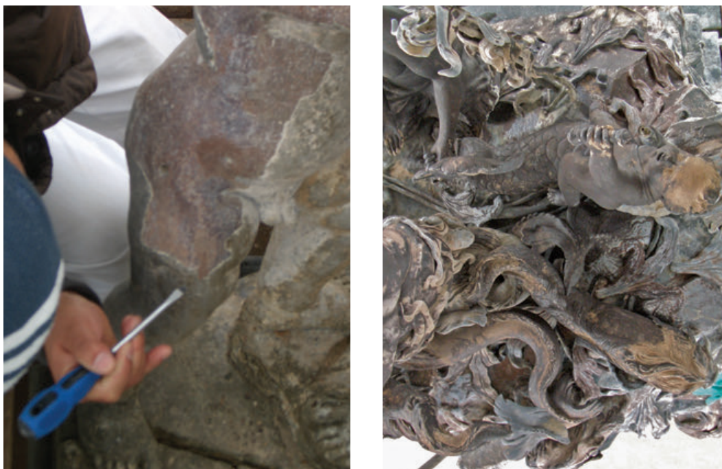
Figure 7. Concretions and patinas in the lead sculptures. Left: detail of the mechanical removal of the whitish concretion that covers the reddish patina formed on the dolphin of the Malta Fountain. Right: detail of the complex decoration of the central block of the Neptune Fountain showing the wide variation in color acquired by the lead surfaces, ranging from gray through reddish to nearly black areas, depending on the water flow over them, apart from the evident concretions on the most exposed parts.
