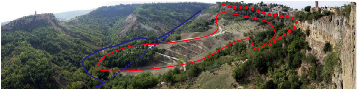
Figure 3. Area of the landslide of 1114 along the side of Lubriano. Red dots: ring area; red line: body of the landslide; blue broken line: former route of the stream Lubriano; continuous blue line: present course of the stream Lubriano
