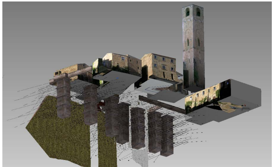
Figure 8. 3D rendering of the complete intervention, showing the position of the cavity wells
