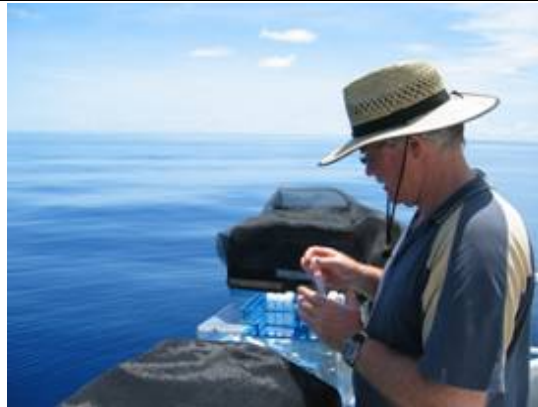
Fig. A7 Preparing water samples for incubation to measure plankton production in water baths designed to simulate the light climate at discrete depths in the water column.
