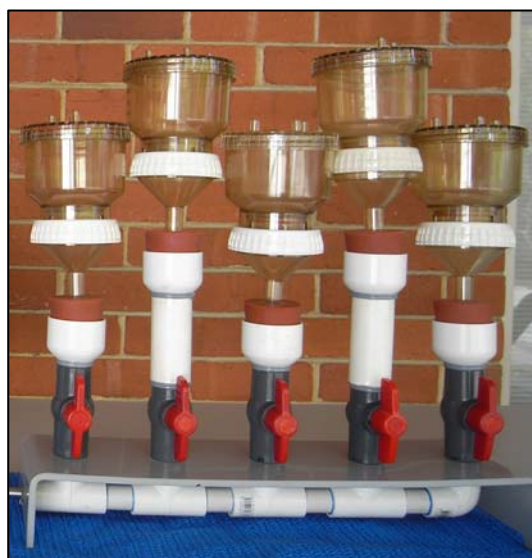
Fig. 6 Sediment filtration manifold
