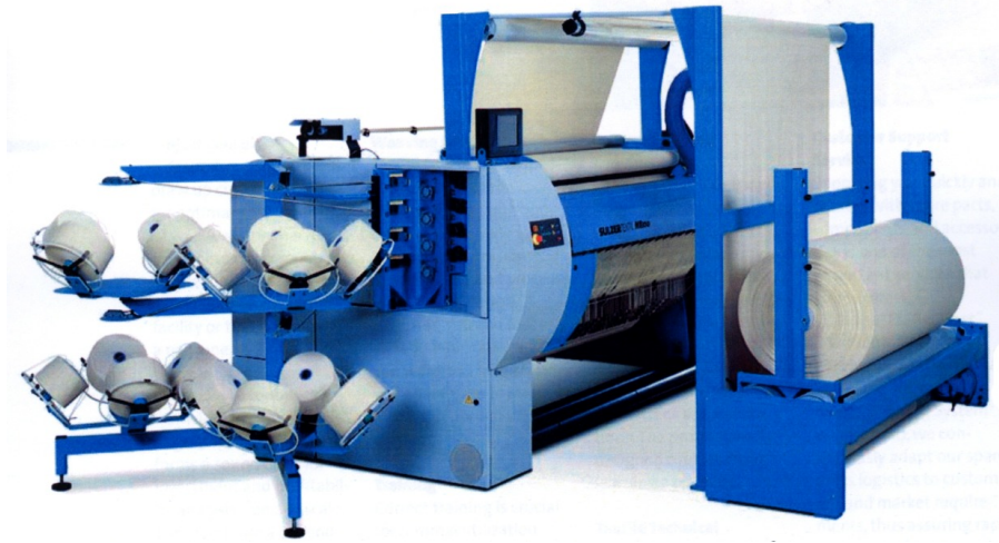
Figure 18.20 Multi-phase weaving loom. Source: Sulzer Textil.
