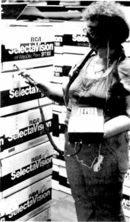
Fig. 4. Portable bar-code reader. The operator is using a portable bar-code reader to record the serial numbers of completed players being shipped to the warehouse. The information is stored in the reader memory (a maximum of about 500 fourteen-digit numbers can be stored). The reader will later be connected to the computer interface so that the stored information can be transferred to the computer data base.
