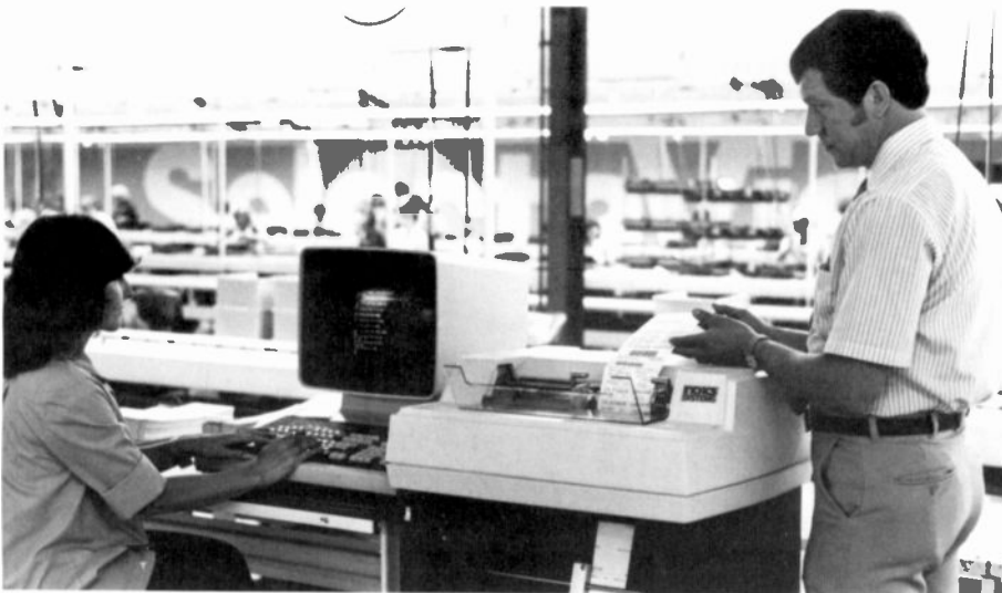
Fig. 5. Label printer and CRT terminal. This label printer, which is driven by the computer, is one of two located in the manufacturing area. It is used to print instrument multi-part labels, subassembly-ID tickets, and test-and-repair code charts. All of these tickets and charts contain bar codes, corresponding numbers, and other information. The CRT terminal is used to transmit the required parameters of the tickets and charts to the computer, and it can be used for systems operations as well as for displaying reports.
