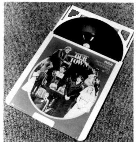
Fig. 3. VideoDisc caddy. Because of the very small dimensions of the recorded information, the disc is kept in a protective plastic sleeve, or caddy, at all times except when being played in a player. The plastic frame surrounding the disc, called a spine, serves to move the disc into and out of the protective sleeve when the disc is inserted into and retrieved from a player.
