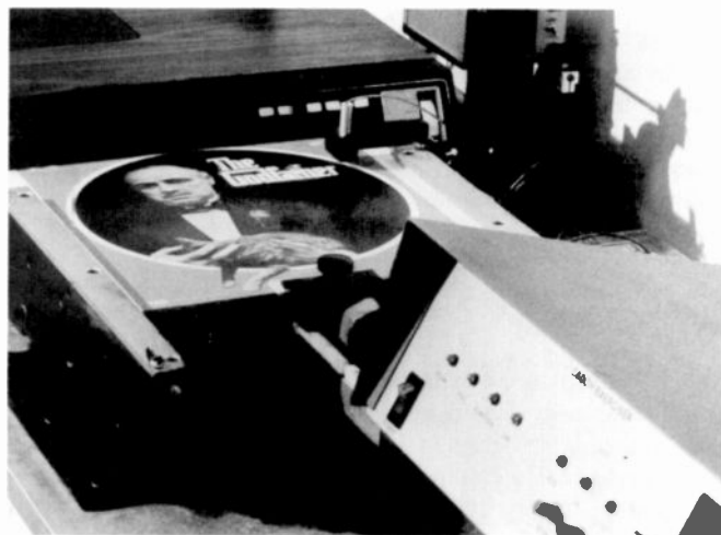
Fig. 1. Caddy exerciser for player life-test cycling.
