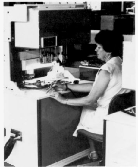
Fig. 2. Automated test equipment. This automated tester is one of several that align and test the major printed-circuit boards of the VideoDisc player. It transmits the test results directly to MACS.
