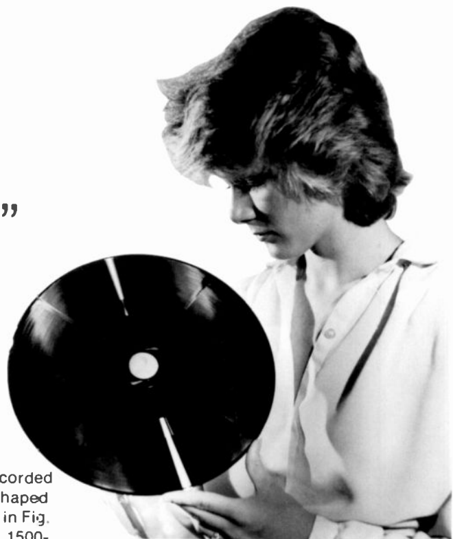
Fig. 1. The VideoDisc is 12 inches in diameter and 70-mils thick. The TV signal is recorded in a spiral groove—10,000 grooves per inch—about 40 times as many as on an audio-LP record. The disc material is made electrically conductive by the addition of 15 percent of finely divided carbon. In playback, the disc rotates at 450 revolutions per minute.
