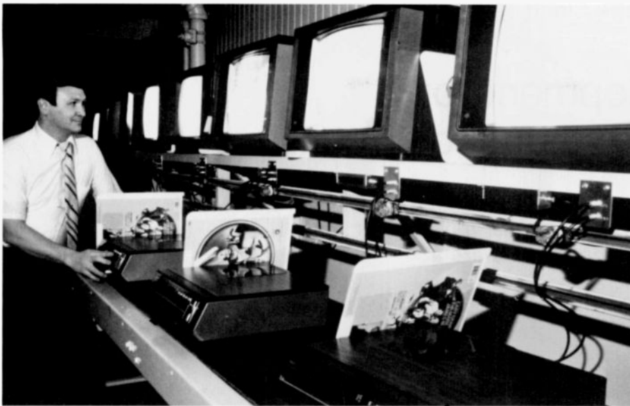
Fig. 2. Consumer Acceptance Laboratory (CAL) tests being performed on part of the player sample taken from the daily production.
