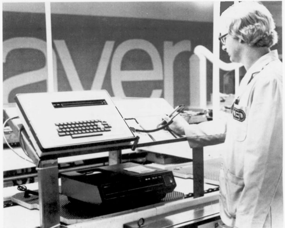
Fig. 3. Bar-code reader. This bar-code reader is one of several located on the manufacturing line. It is used to transmit instrument serial numbers, test codes, and repair information via bar code to the computer. It transmits part legends and operator numbers via keyboard.
