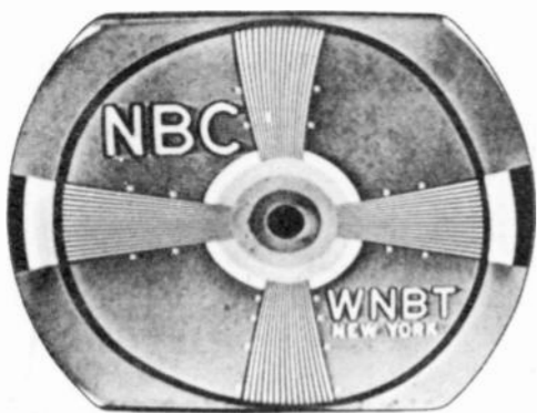
Figure 25—Horizontal Drive Control Misadjusted
