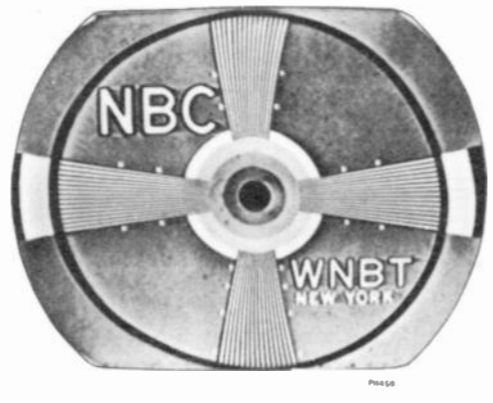
Figure 21—Horizontal Linearity Control Misadjusted
