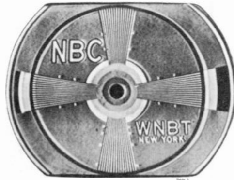
Figure 25—Horizontal Drive Control Misadjusted
