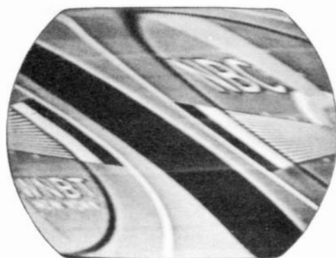
Figure 27—Test Pattern Showing Out of Sync Condition When Horizontal Hold Control Is in a Counterclockwise Position—Just Before Pulling In Sync
