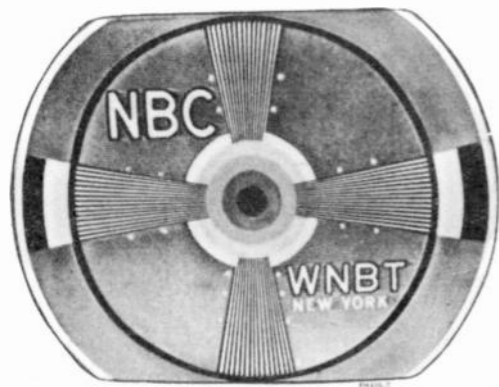
Figure 22—Focus Coil and Ion Trap Magnet Misadjusted
