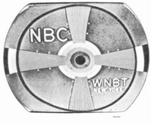
Figure 23—Horizontal Drive Control Misadjusted
