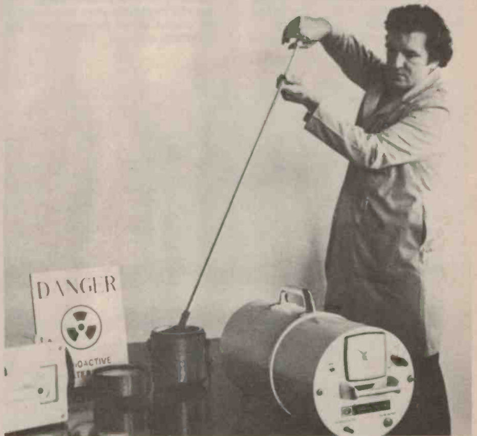
The operator uses long tongs to keep his body away from the radioactive material in the container, whilst the monitor continuously checks the radiation level. (Courtesy Nuclear Enterprises Ltd.)
