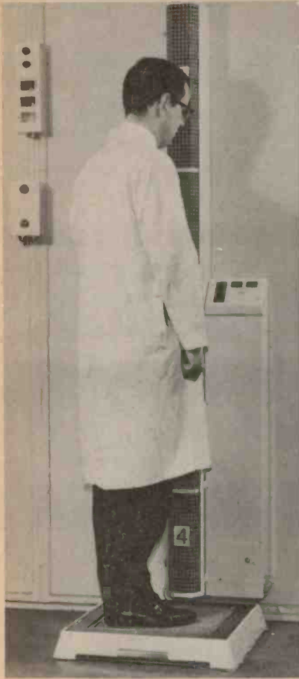
Monitor for checking the contamination of personnel working with radioactive materials. It comprises a vertical array of 11 beta/gamma Geiger detectors with an additional detector for monitoring the soles of shoes. An alarm bell is included in this equipment, whilst the tone chimes sound when there is no contamination. (Courtesy: Nuclear Enterprises Ltd.)
