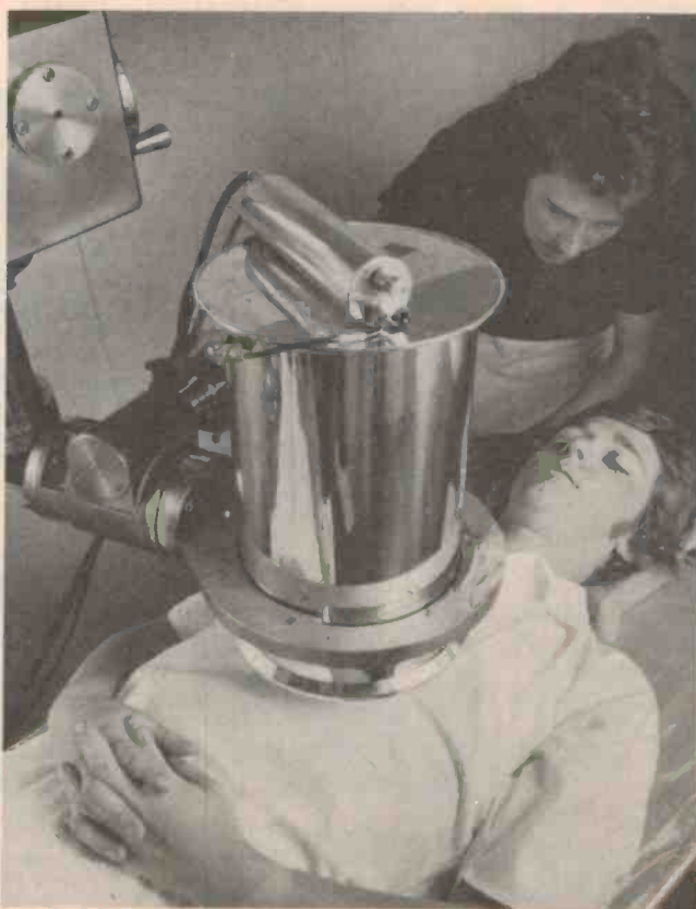
Measurement of lung contamination by plutonium-239. Apart from alpha particles, this isotope emits low energy gamma rays which penetrate the chest wall and are detected. (Courtesy: U.K.A.E.A.).
