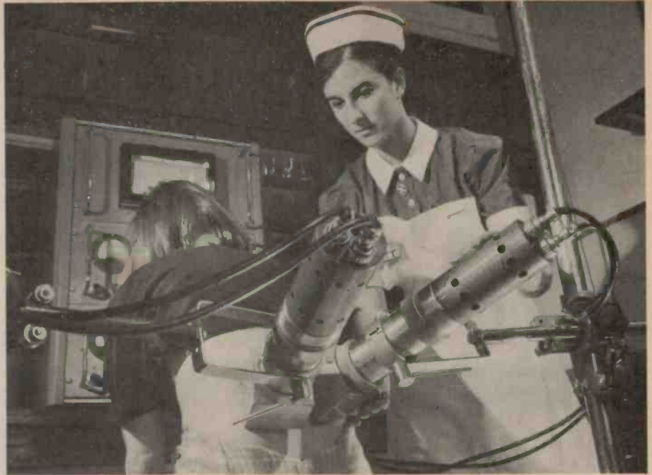
The patient has been given an injection of a radioactive material which is rapidly excreted by the kidneys. The two detectors, one behind each kidney, drive the pen recorder above the patient's head which produces a chart containing kidney function information. (Courtesy: U.K.A.E.A.).
