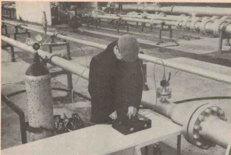
Calibration of the reference flow meters at the Gas Council's Engineering Research Station at Killingworth. Ethyl bromide containing the radioactive isotope bromine-82 is employed. (Courtesy: Gas Council and U.K.A.E.A.).
