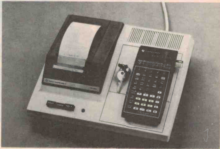
Fig. 2. The PC100A allows printing of results, headings, prompts...
