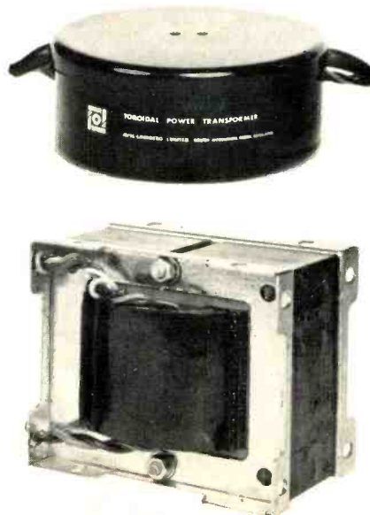
Fig. 2—The physical advantages of toroid transformers are demonstrated in this photograph of a 90-VA toroid transformer compared with a similarly rated conventional transformer. The toroidal transformer is 1.8 in. H and 4.2 in. diameter, with a weight of 3 lbs.; the conventional transformer is 3½ in. H x 3½ in. L x 3½ in. W.
