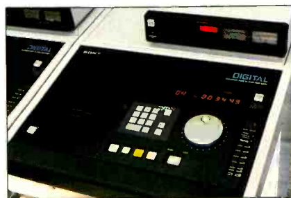
Several computer systems were set up to generate music, either by reading magnetic stripes or by keyboard commands, as with these systems from NEC (left). Sony's CDP-5000 Compact Disc Player is intended for pro use and can locate by track, time or frame (below).
