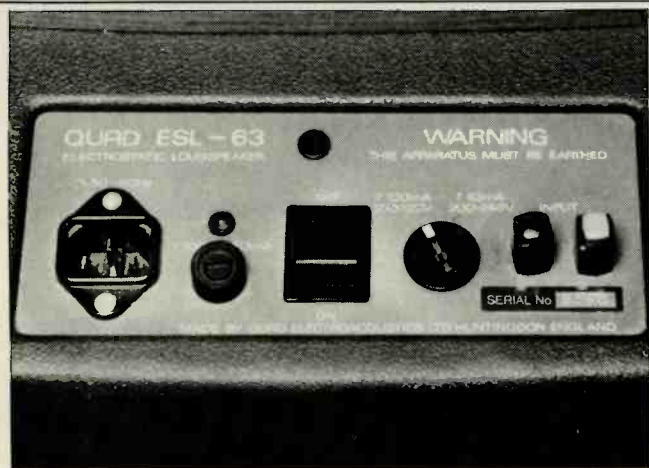
Grouped at the speaker's base are the power leads, fuse, on/off switch, voltage selector, and input terminals.
