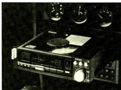
Now you see it, now you don't. The Philips CD10 slides into the dash after loading—or comes out, for portable use.
