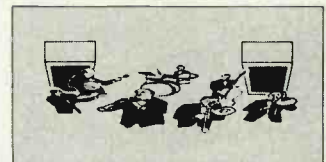
Conventional stereo: The sound is heard, more or less, on a flat curtain of sound between the two speakers. Volume differences only. The timing cues are gone.
