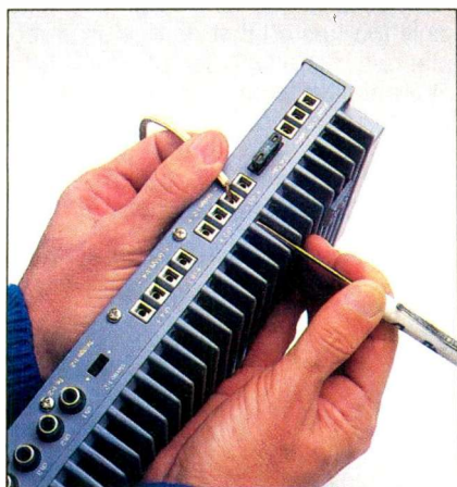
The screws for the ADS's speaker and power connections are concealed between the unit's heat-sink fins.
