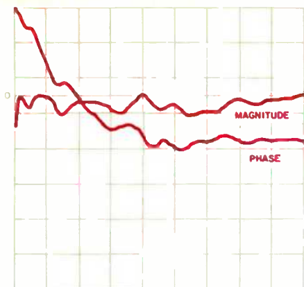
Fig. 4 —Phase and magnitude plots vs. frequency. The vertical scales are 6 dB/div. for magnitude and 45°/div. for phase.
