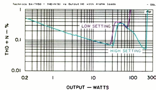
Fig. 5—Stereo THD + N vs. output for 8-ohm loads (A) and at 1 kHz into 4-ohm loads for high- and low-impedance settings (B).
