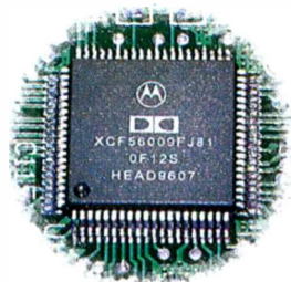
B&K's new surround sound components are powered by the 24-bit Motorola 56000 DSP.
