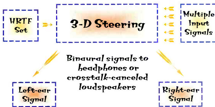
Fig. 3—By digitally processing head-related transfer functions (HRTFs), it's possible to electronically synthesize the left- and right-ear signals appropriate for any direction.
