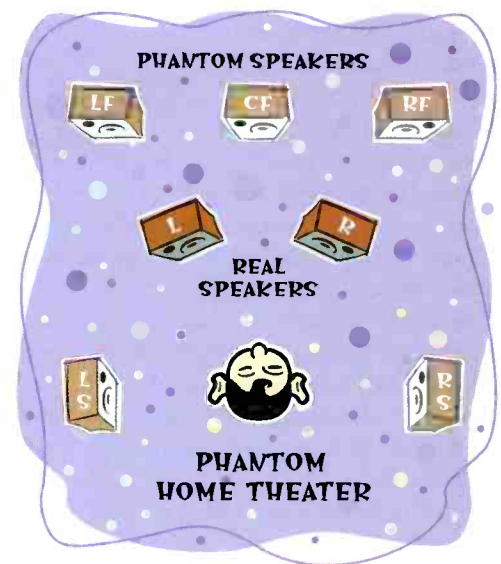
Fig. 5—Speaker-based binaural synthesis can create multichannel sound reproduced through five phantom speakers but actually generated by just two real speakers.
