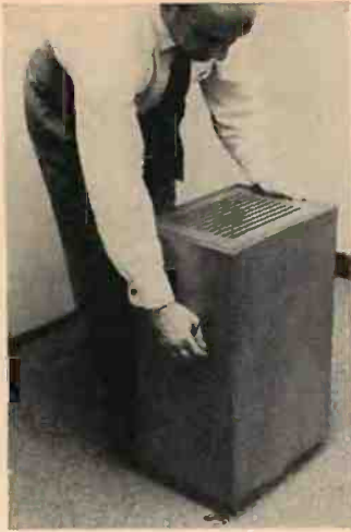
Volume control and switches of the Royce "Stereo-Rama" are located on its side, with the sound emerging from slotted top.
