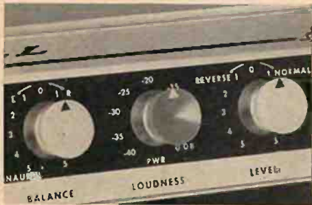
New features of the Bell Model 3030 Stereo Amplifier include Single-Knob Balance Control, Continuously Variable Loudness Control and Level Control with Built-In Channel Reverse for Stereo.
