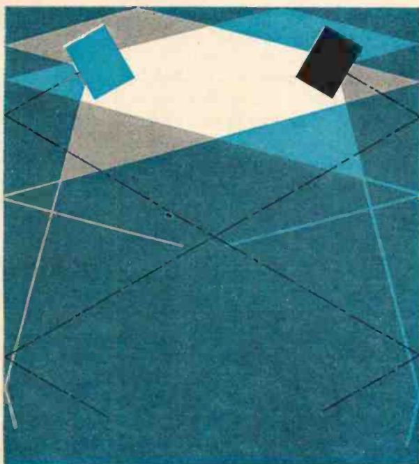
Reflected sound, obtained by angling speakers toward walls, increases overlap and overall sound diffusion.
