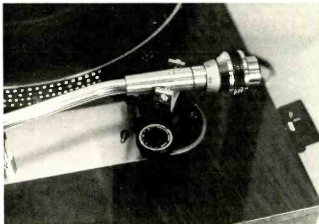
The pivot area of the precisely machined tone arm incorporates the anti-skating adjustment and damped cuing lever.
