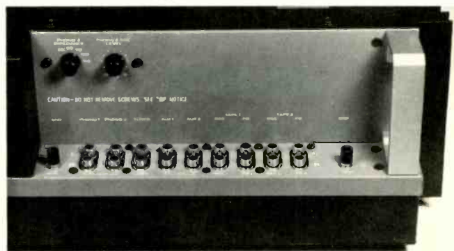
The right and left side panels of the Pioneer SA-9900 incorporate a section that provides a convenient mounting surface for the profusion of input and output terminals. Two switches above the phono-input jacks select phono-input load impedance and phono or mic level.
