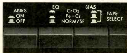
Automatic Noise Reduction System reduces tape hiss.
