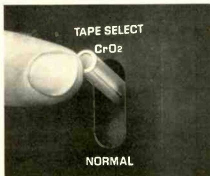
The chrome position on the tape selector is designated differently on different machines: CrO 2 , Chrome, Special, SX, Position 1, High or 70 \mu s.
