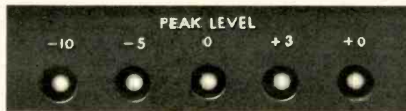
5 LED peak level indicators help eliminate distortion.
