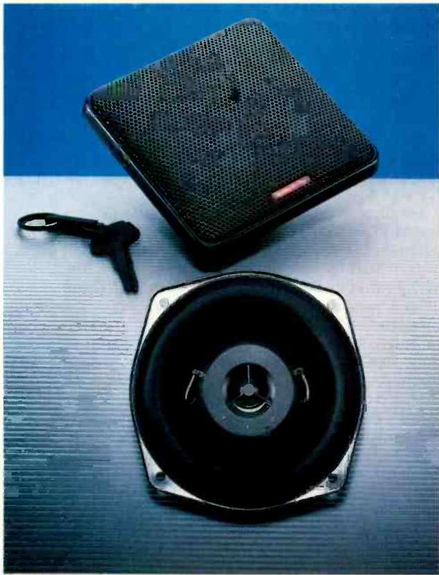
The Model 757 "uniaxial" speaker from Boston Acoustics combines a 5¼-inch long-throw woofer and a ¾-inch wide-dispersion tweeter. Frequency response is 58 to 20,000 Hz \pm 4 dB. Both drivers use weatherproof copolymer diaphragms. Price: $119.95 a pair.
