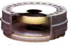
Also, other headphones use the same driver for the highs and lows so they have to compromise between the massive movements for low bass and the fine vibrations of the highs.
