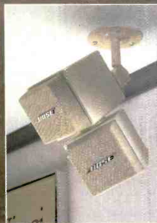
You can mount the arrays from the ceiling, much like track lighting.
