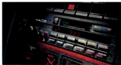
A 200-watt Audi/Bose system featuring eight speakers, including a bass module, and a Blaupunkt-made cassette tuner (above) is optional in the 1994 Audi 100S station wagon.
