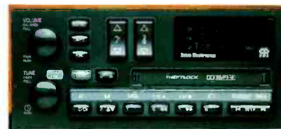
A Delco cassette receiver equipped with an RDS decoder that receives special text and audio broadcasts (traffic reports, etc.) will be offered as an option in GM vehicles next spring.
