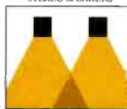
Box Speakers offer only a small stereo hot spot where true stereo sound can be enjoyed.
