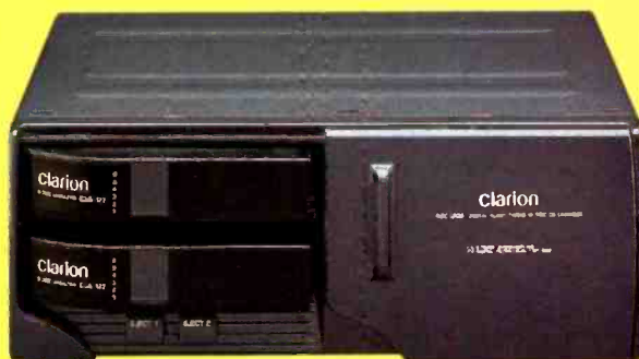
Clarion's RDC1205 CD changer ($390) accepts two six-disc magazines and has a circuit that mutes hiss between tracks.
