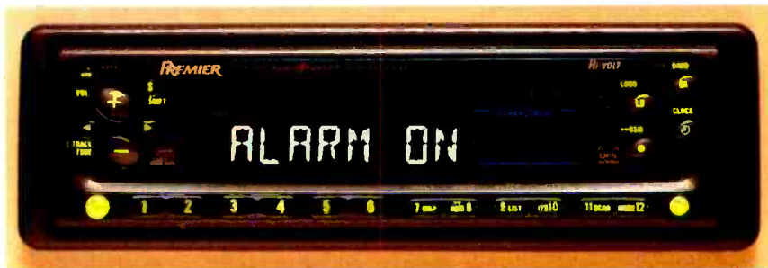
A Detachable Face Security (DFS) system in the DEX-P88 ($630) and other Pioneer Premier source units generates an ear-piercing tone to ward off intruders.
