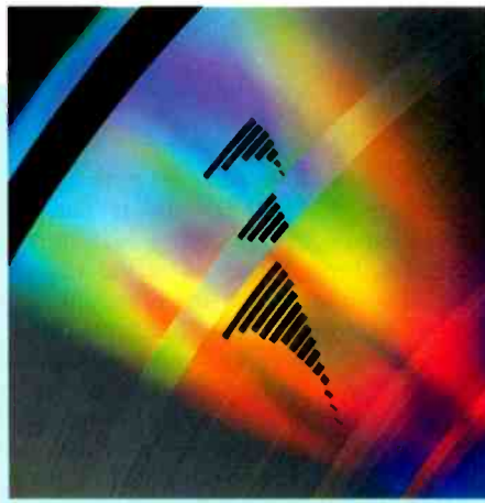
Simulated disc damage on the Pierre Verany test disc. We use the bottom-most wedge.
