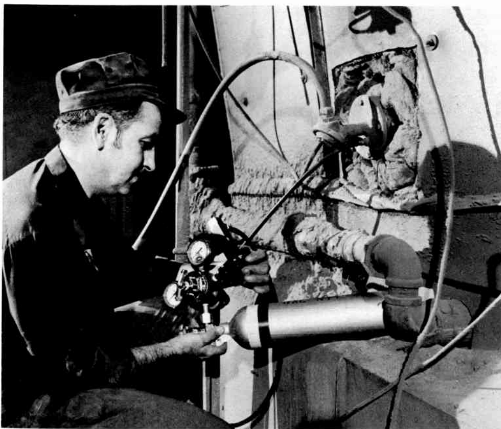
6—The Oxygen Analyzer can be supplied with provisions for recalibrating it without removing it. A gas mixture with a known percentage of oxygen is passed through a tube to the cell, and the resulting output is compared with the known oxygen percentage in the mixture.
