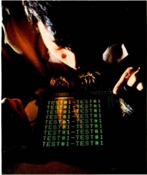
Above —Each electroluminescent cell can be energized without activating other cells in the same row or column.
