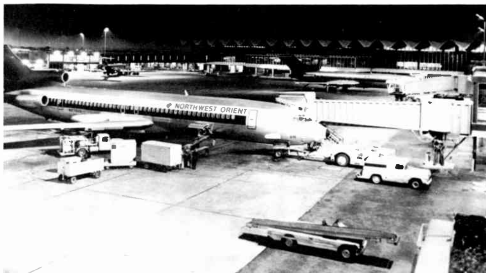
Modern HID lamps were first applied outdoors, and that is still a large application area because of their long life and high efficacy. Metal-halide lamps were chosen to illuminate loading areas at Minneapolis/St. Paul International Airport.
