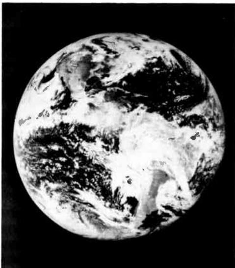
Views of the western hemisphere with its weather patterns are transmitted from the SMS-1 satellite and recorded at ground stations by laser-beam recorders. A picture can be made every half hour for close monitoring of weather movements.
