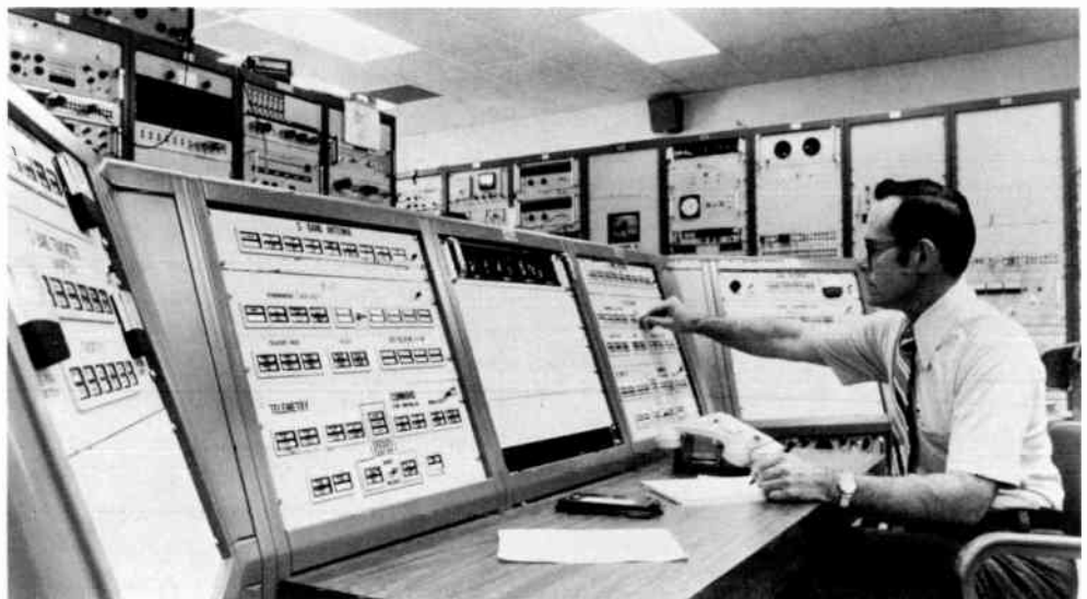
This equipment provides the means for controlling SMS satellites and for acquiring, synchronizing, and stretching the data received from them. It is located at NOAA's Command and Data Acquisition Station.
