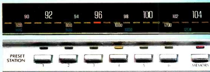
The digital circuitry ensures that every station received is automatically locked in for lowest possible distortion, with its frequency indicated both on a digital readout and by a LED indicator along an analog type dial.
