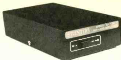
The BA-26 head amp is designed to boost the signal from a 980 LZS to a level high enough to drive standard phono inputs.
