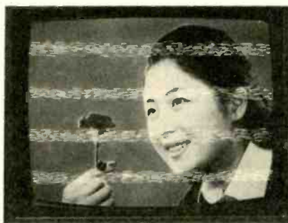
Using Betascan, you can vary the fast-forward speed between five- and twenty-times normal—and still see a picture while so doing. Noise bars are visible, particularly in faster modes, but the picture is clear enough to facilitate easy location of specific points on the tape.
