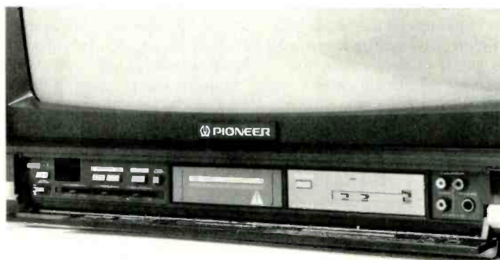
CONTROLS , an extra set of audio-video inputs, a headphone jack, and two slots for special input modules are behind a flip-down door just below the SD-25's screen. The right-hand slot is shown here with the SD-X5 TV tuner in place.
