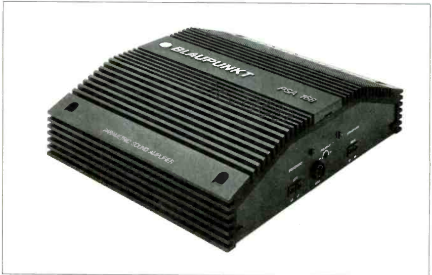
The Blaupunkt PSA-168 power amplifier takes custom equalization modules for specific car models.
