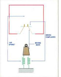
Fig.3: Placing a driver in a sealed box Fig.3: Placing a driver in a sealed box prevents the acoustic short circuit of Fig. 1b but the trapped air volume acts as a spring in parallel with the driver suspension. The fundamental resonance is raised. Driving the cone against this air spring can cause cone breakup in small enclosures and results in a phase lag if the damping factor is poor
