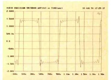
Fig.4: Square-wave response for 7% sample-rate increase through Motorola 55001
