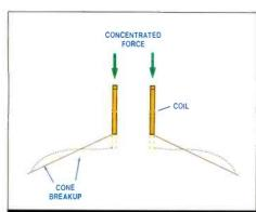
Fig.2a: The concentrated force from a moving-coil motor may distort the cone
