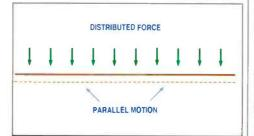
Fig.2b: The electrostatic loudspeaker produces uniform drive over the surface of the diaphragm so there is no tendency for it to break up
