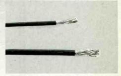
MULTICORE CABLES WITH AND WITHOUT OVERALL SHIELD
