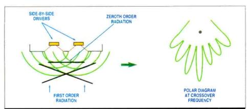
Fig.4: If drive units in a multiway system are wrongly placed side by side, at the crossover frequency when both units contribute to output there will be interference between them resulting in a spiky polar horizontal diagram which impairs the imaging
