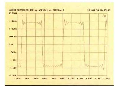
Fig.3: Square-wave response for 7% sample-rate increase through AD 1890
