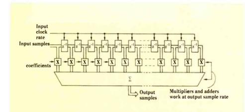
Fig.2: Schematic representation of a finite impulse-response filter
