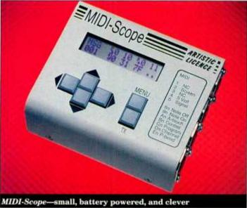
able to test merge, Thru and filter functions on units that perform such roles. Error messages are shown for framing and for overrun errors. The choice of hex or icon display is considerate but I reckon that most users will prefer the latter simply because of its immediacy. Even using icons, the display takes some getting used to because of the number of icons and the amount of data involved and the manual fails to communicate the true potential of this device.
