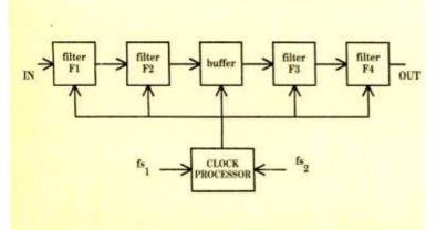
Fig 1: Asynchronous convertor schematic employing multiple digital filter stages
