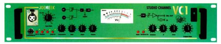
THE LATEST IN a Fletcher ElectroAcoustics range that also includes valve-based units is the VC1 Studio Channel. The unit is a single-channel preamp with a JoeMeek compressor and an enhancer. Needless to say it's still the characteristic shade of automotive paint green that has become the trademark of the JoeMeek stuff. How the colour came about is one of those marvellous accidents of happenstance that deserves to be told.
