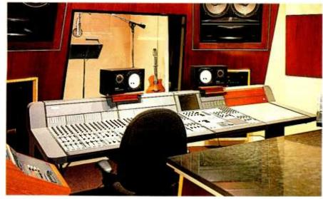
With the Euphonix, every keyboard is normalled into the board and available at the touch of a button.
