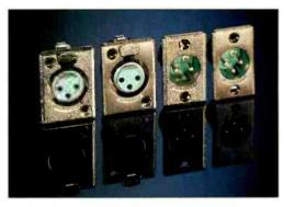
The D series of Q-G® connectors offers a choice of satin, pebbled, or black metal finish for panel or chassis-mounting. Choose from 3 to 7 contacts or pins with silver or gold plating. Shown above, left to right: D3F (pebbled), D3FS (satin), D3M (pebbled) and D3MS (satin). For black finish order D3MB or D3FB
