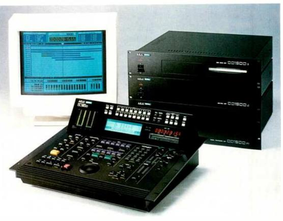
9-pin protocol) master or slave, a time code master or slave (LTC, MTC, VITC) or a biphase master or slave (2, 4 or 10 cycles/frame). The unit can be synchronised to; wordclock,PAL-SECAM or NTSC video, digital audio or internal clock.
