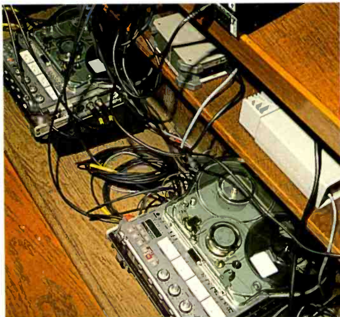
Hiding in the Queens College Pews—sync'd Nagra-Ds running at 24-bit, 96kHz
