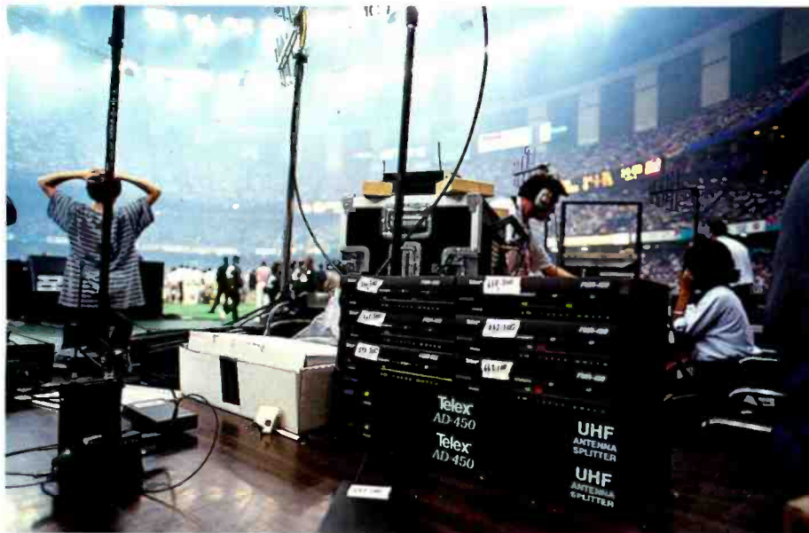
Telex telecomms rack at the pitch in New Orleans—match referees used PH1 and PH2 headphones, FMR450 and SoundMate systems were used by the players
