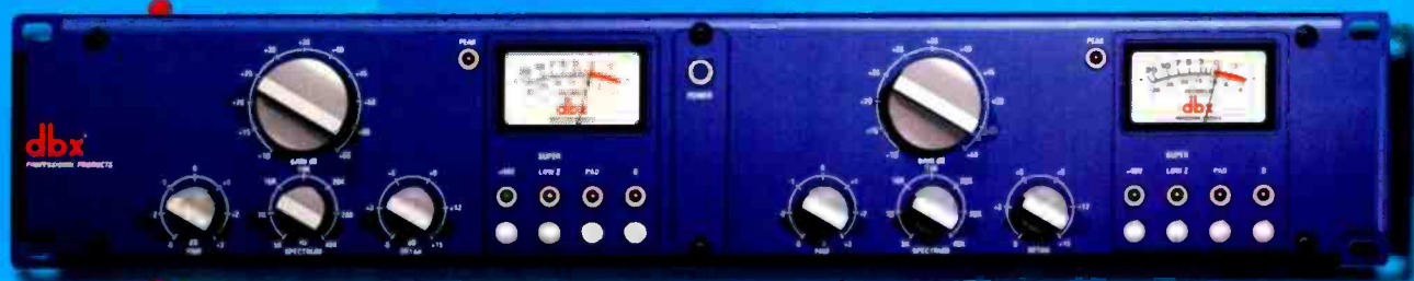
The new dbx V8 is based on the David Blackmer deci-linear VCA. Featuring 127db dynamic range and sounds very transparent.
