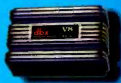
The new dbx V8 is based on the David Blackmer deci-linear VCA. Featuring 127db dynamic range and sounds very transparent.
