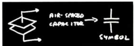
Fig.3: What is a capacitor?
