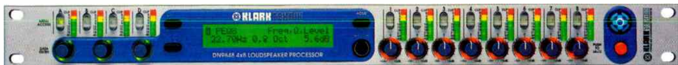
Klark Teknik's DN9848 loudspeaker management system includes a digital processor.
