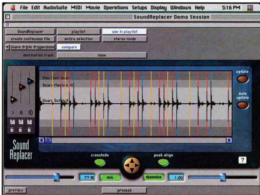
SoundReplacer loads up to three samples simultaneously (represented by color-coded trigger points and fader controls).
