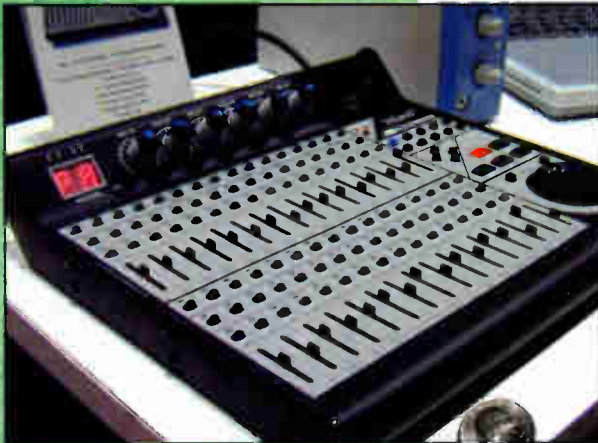
JLCooper's CS-32 MiniDesk brings 32 DAW channel control strips and tape-style transport keys with jog/shuttle wheel to a notebook-sized worksurface. Note the quarter at lower right and Digidesign M-Box in background to help show product's scale.
