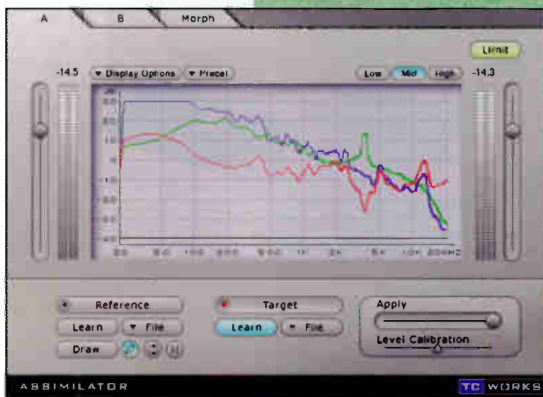
TC Works' Assimilator plug-in analyzes a reference mix and then applies that EQ curve to new material.
