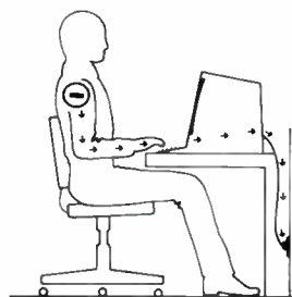
(Above) Static charges discharge to ground directly through delicate microelectronic circuitry, and (below) field induced charges cause slow degradation of integrated circuits.
