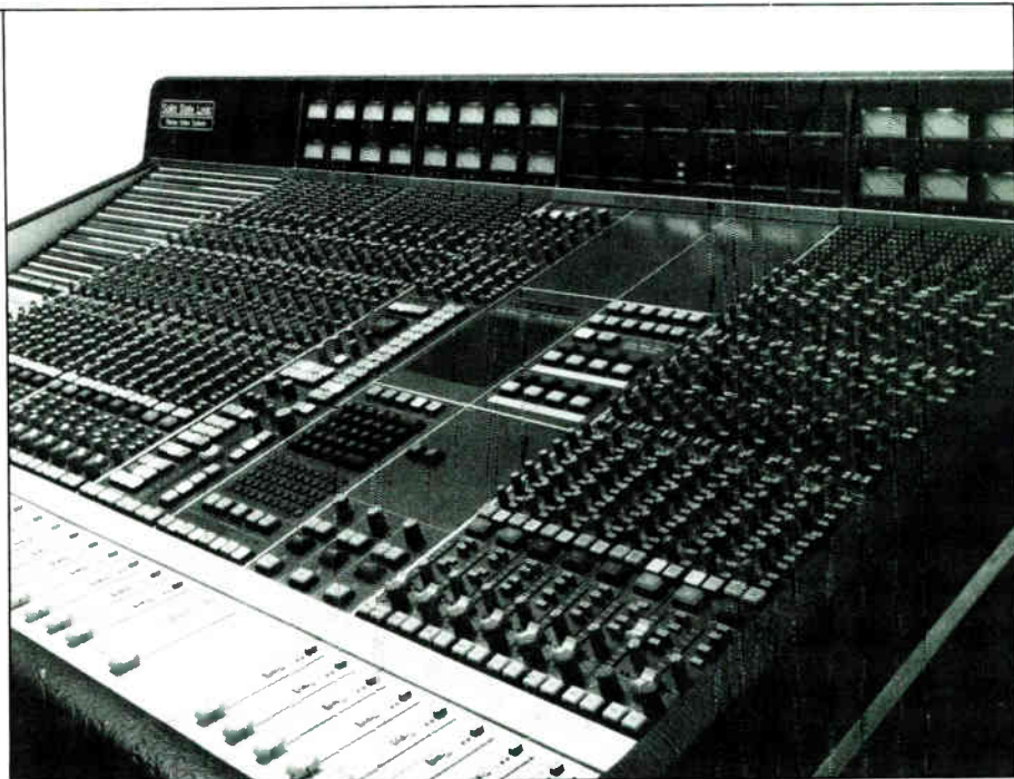
The Solid State Logic SL6000 E console incorporates a comprehensive computer automation system for the control of both console and transport functions.
